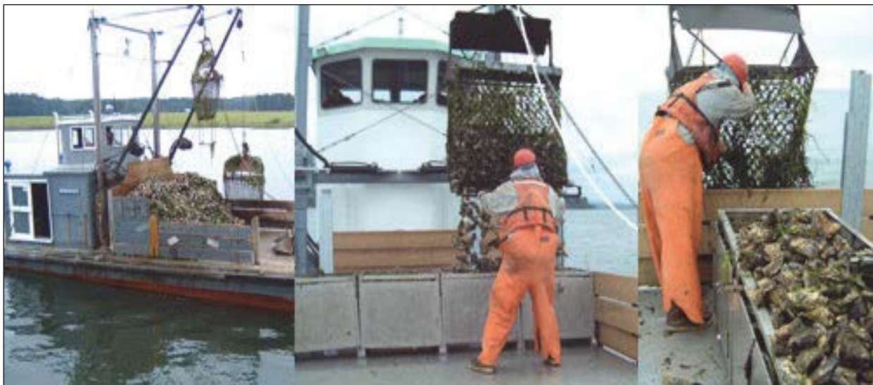
Figure 15. Oyster dredge with boom cranes and bags (Corps 2015, p. 19)
